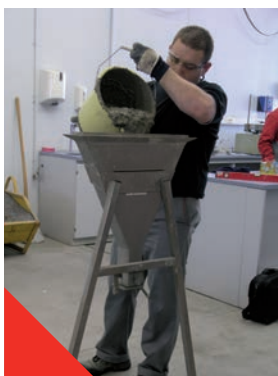
Fig 3.2.3 Essai V Funnel
