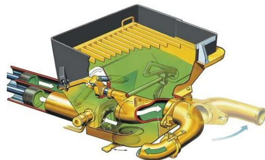
Figure 10: Putzmeister S-Valve cutaway
