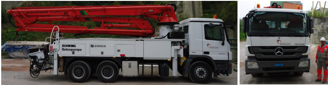
Figure 8: Truck mounted concrete pump
