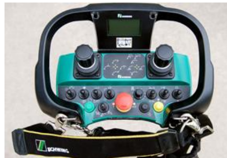
Figure 29: Schwing remote control unit with emergency shut-down button
