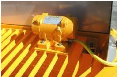
Figure 9: Hopper grate & vibrator
