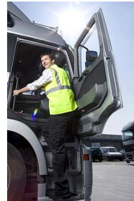
Figure 16: Three-point contact for access & egress
